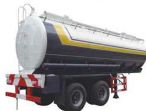
2 axles 40CBM liquid chemical tank semi trailer
