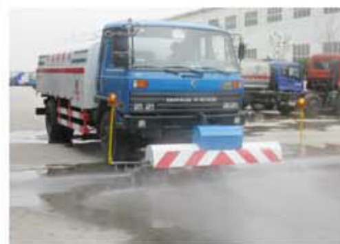
Dongfeng road flushing truck, 8m3 tank, 170hp
