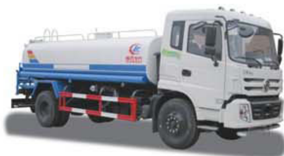
Sinotruck, Engine 336/371HP,Volume : 16m3
