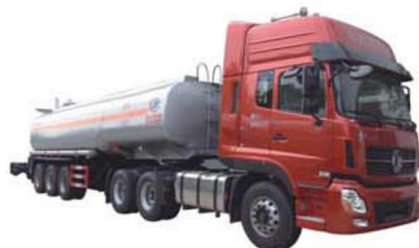
3 axles 48CBM fuel tank semi trailer
