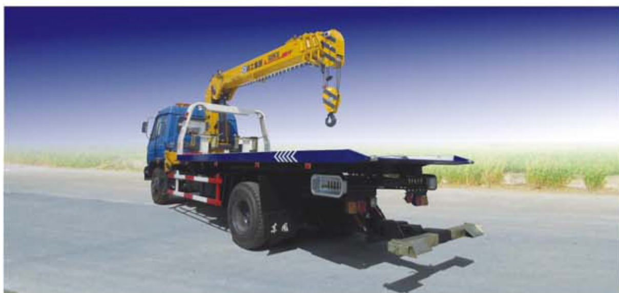
DONGFENG wrecker truck with crane 5ton-8ton
