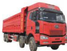
Brand:FAW 8*4 LHD/RHD Engine: 340HP, 350HP, 380HP Loading Capacity: 35T - 45T
