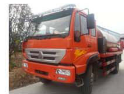
Sinotruk 9-10m 3 , 190HP Asphalt distribution truck
