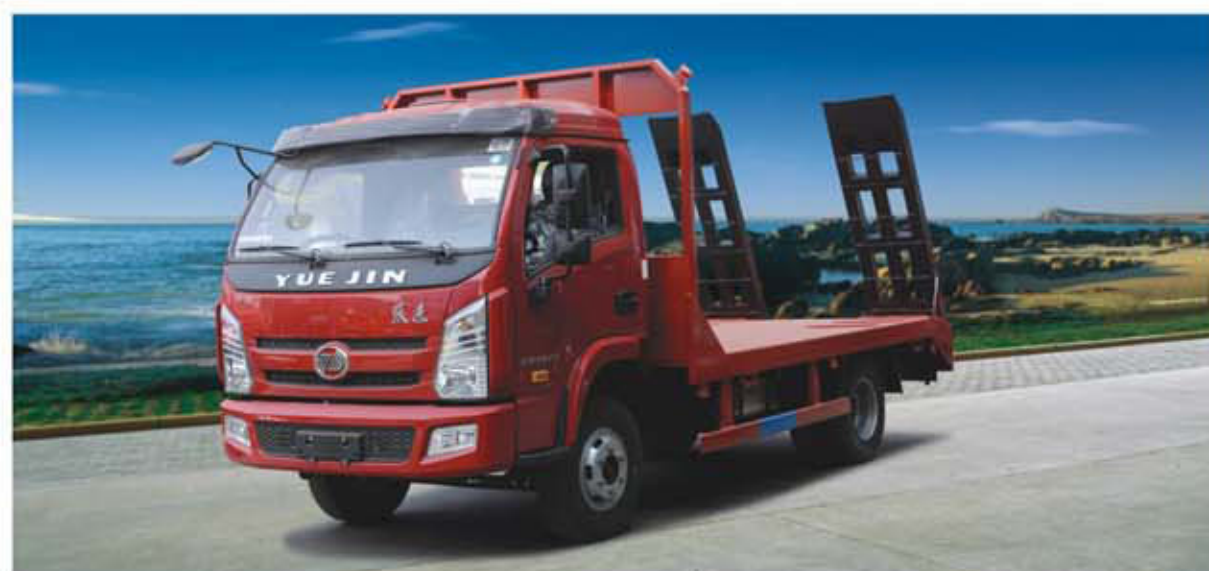
Yuejin Self loading truck (90HP-130HP,6-8 tons,flatbed length:4.7m )
