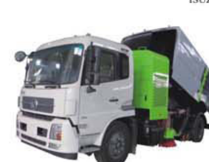
Dongfeng cleaning sweeper truck, 7m3 dust tank & 3.5 water tank
