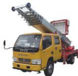
Brand : Dongfeng 4*2 LHD or RHD Engine: 95HP Working Height :20-28m
