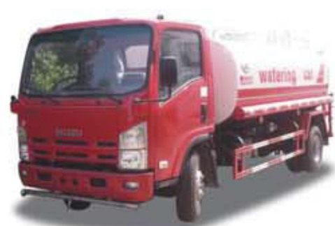
ISUZU water tank truck,engine:ISUZU 190hps, volume:6-8CBM
