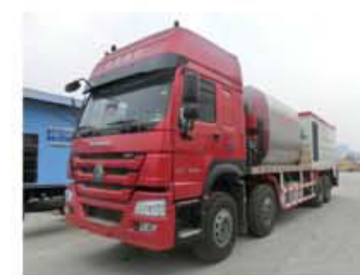
HOWO 8*4 synchronous chip sealer 10m 3 asphalt tank+16m 3 chip tank
