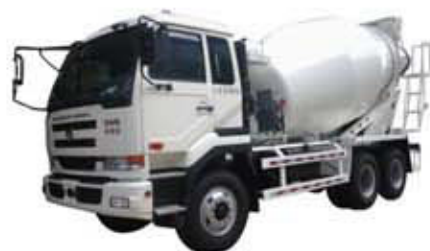
Brand: Dongfeng 6x4 LHD or RHD Engine: 310HP, 350hp, 380hp Volume: 6 cubic meter to 12 cubic meter
