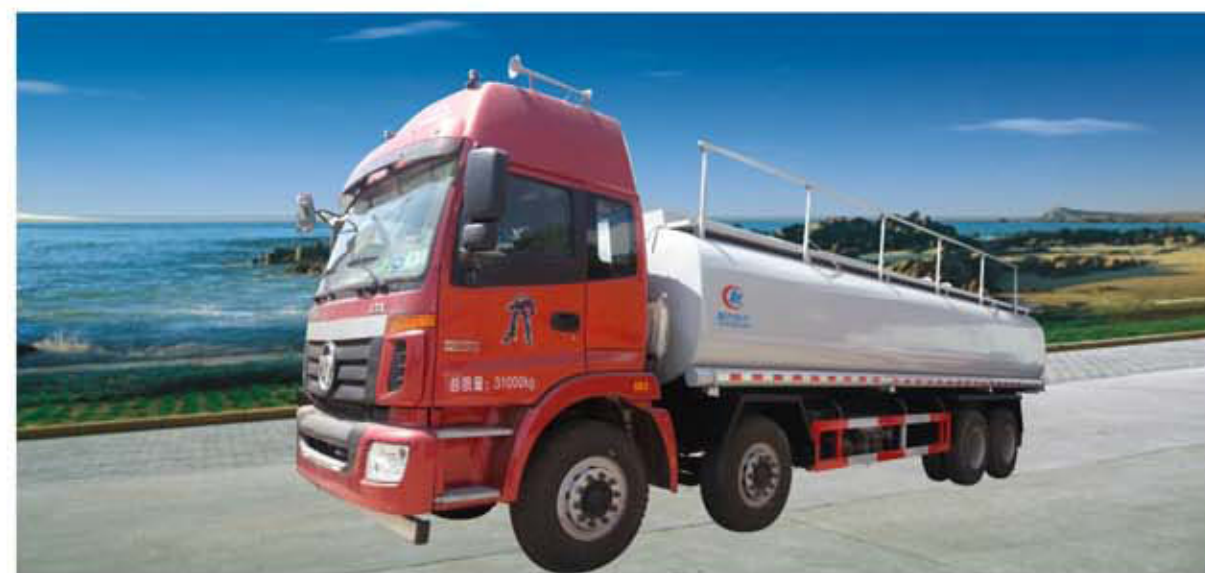
FOTON 8x4 chassis, 290 hp , 30-35cbm fuel tank
