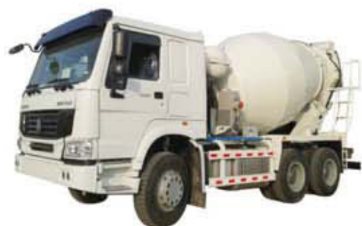
Brand: SINO HOWO 6x4 LHD or RHD Engine: 266HP, 290HP, 336HP, 380HP Volume: 6 cubic meter to 12 cubic meter
