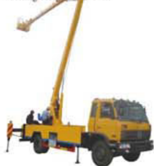
Brand :Dongfeng 4*2 LHD or RHD Engine : 170HP Working Height :10-16m
