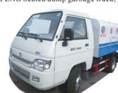
DONGFENG Sealed dump garbage truck, CHAOCHE engine 95hp, 4-5m³
