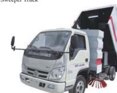
Foton 1.5 water tank & 3-4 m3 dust tank
