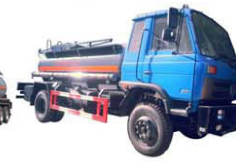
Dongfeng 4x2 chassis, 190 hp , 10cbm chemical tank for caustic soda
