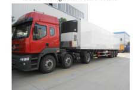
3 axles 40 feet Refrigerator trailer with Carrier units
