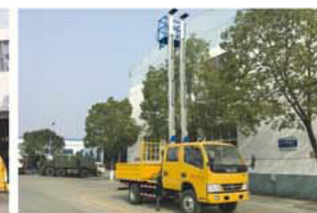
Aluminum alloy vertical lifting aerial working vehicle
