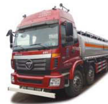
FOTON Auman 8x4 chassis,cummins 270hp, 25-30cbm Aluminum fuel tank
