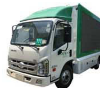
Forland, Engine: 125hp, LED Screen: Double Sides P6 with Banner Roller
