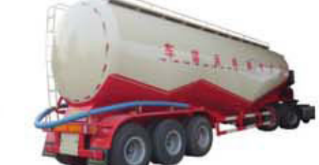
Brand: CLW Type:double V type trailer Volume:30m3 to 80m3
