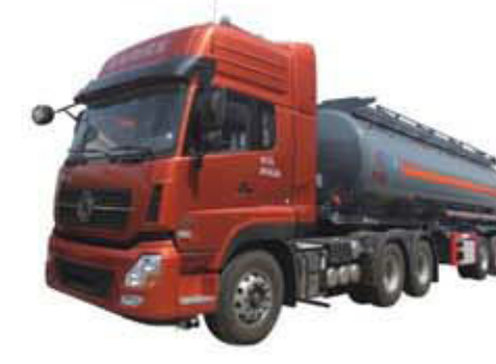
3axles Chemical tank trailer, 30cbm sulphuric acid tank
