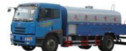
FAW high pressure sewer flushing vehicle, 10m3 tank
