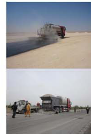
Howo 6*4 asphalt distribution truck, 10m 3 -12m 3 , Intelligent automatic control /half automatic control
