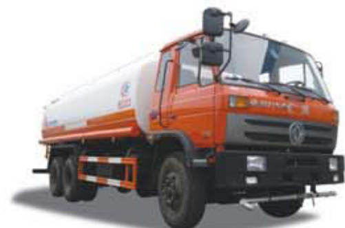
Dongfeng water tank truck, engine:Cummins 210hps, volume:18-20CBM
