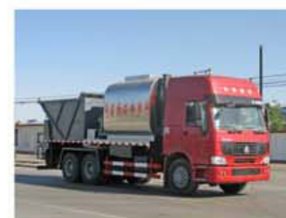
HOWO 6*4 synchronous chip sealer 8m 3 asphalt tank+12m 3 chip tank
