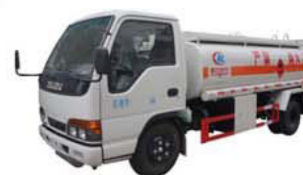
ISUZU 4x2 chassis, 98 hp , 3-5cbm fuel tank, fuel dispenser truck
