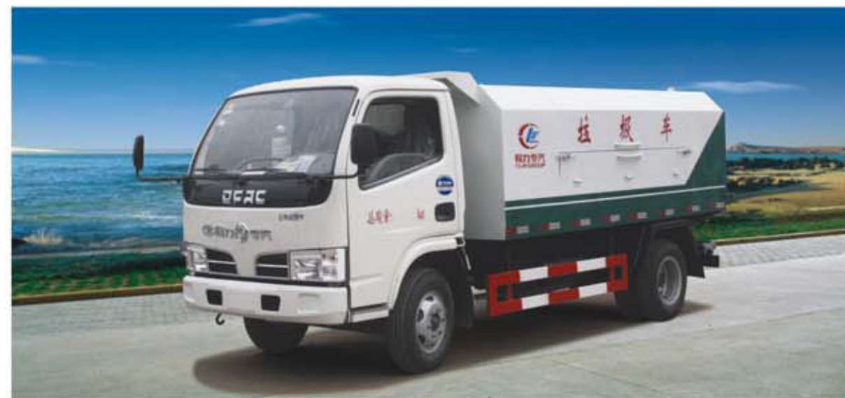
DONGFENG Sealed dump garbage truck, CHAOCHE engine 95hp, 4-5m³
