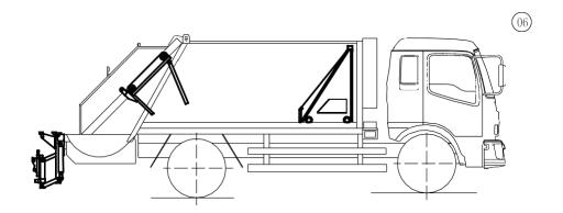
Step 7. Turn the negative pressure operation knob to the left recovery position, recover the negative pressure plate, release the knob back to the median, and complete one load of garbage, as shown in Fig
