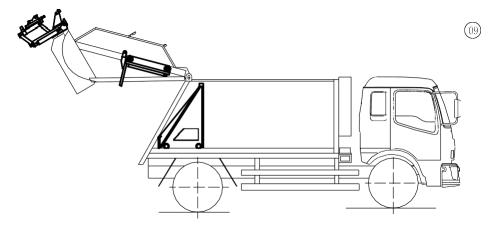
Step 10. Rotate the push plate operation knob to the left recovery position, the push plate is retracted, release the knob; then rotate the bucket operation knob to the left fall position, the bucket is down and locked with the chassis, release the knob, and release the force collector (if the bucket mechanism is the down position), when the vehicle is move. The position of the vehicle is moved as shown in Fig
