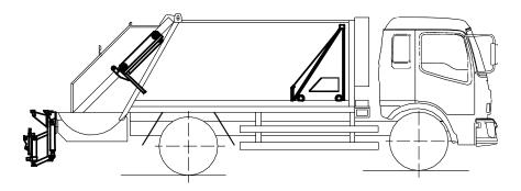
Step 6. Rotate the negative pressure operation knob to the right launch position, the garbage is pushed into the chassis by the negative pressure plate, release the knob back to the median; as shown in Fig
