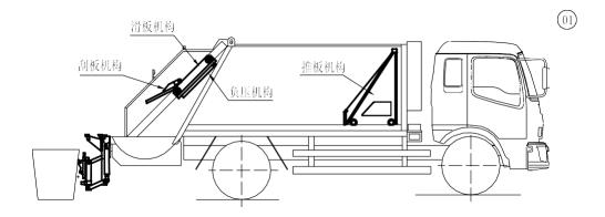
Step 2. Hang the trash can, rotate the bucket operation knob to the top right flip position, the trash can up, garbage automatically into the arc bucket, release the knob to return to the median; as shown in the figure
