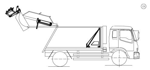
Step 9. Rotate the operation knob of the push pad to the right launch position. Please push the garbage into the car compartment and release the knob to complete the unloading work; as shown in Fig
