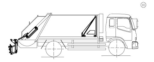
Step 4. Rotate the scraper operation knob to the left scratch position, scrape the garbage along the arc bucket, release the knob back to the median; as shown in Fig
