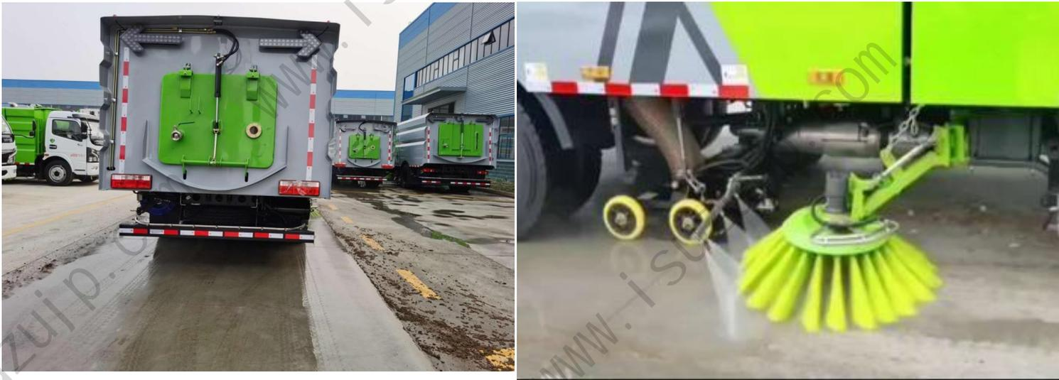
**Working principle:** The auxiliary engine drives the hydraulic oil pump, the high-pressure water pump and the fan to work. The hydraulic oil pump drives the left and right sweeping discs to extend, lift and rotate. The left and right sweeping brushes sweep the garbage on both sides to the front of the suction disc driven by the rotation of the sweeping disc. Pipeline control valve, etc.
