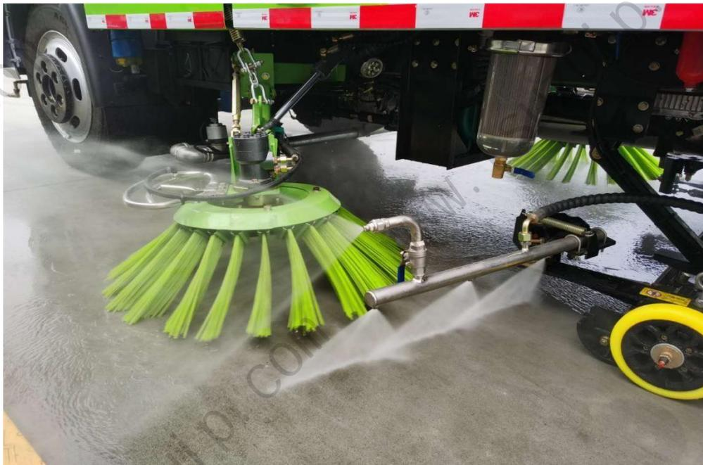
**3. Rear spray foggy dust reduction:** There is a spray boom under the dust bin at the rear of the sweeper, which is equipped with multiple spray nozzles.
