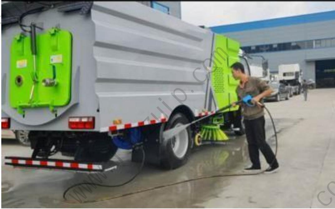
**6.Truck front spot flushing device:** Driven by a high-pressure water pump, it can cooperate with the cleaning operation. In the early stage, the fixed-point dirt on the road can be washed and cleaned, and the dust can be avoided during the cleaning operation. It can also be used with low-pressure flushing operations on relatively clean roads to reduce dryness of the road surface.
